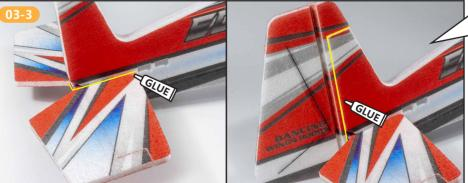
尾翼用泡沫胶粘固。同时调整机翼与机身垂直。 Stick the tail wing with foam glue. Adjust the wing to be perpendicular to the fuselage at the same time.
