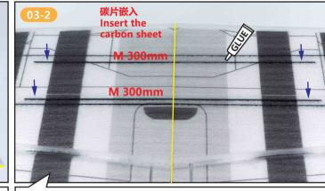
两片机翼对粘在一起,并在图示位置嵌入碳片,用泡沫胶粘固。 Glue the two wings together and embed carbon sheets in the position shown n the figure, finally use foam adhesive to fix.
