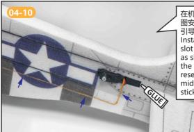
在机身尾部舵机槽内安装舵机,如图安装,舵机线埋入预留槽内,并引导到机身中部。用泡沫胶粘固。Install the servo into the servo slot at the rear of the fuselage as shown in the figure.Embed the servo cable into the reserved slot and guide to the middle of the fuselage,finally stick with foam adhesive.
