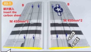
在机翼预留槽埋入碳片,并在图示位置涂抹泡沫胶。左右机翼相同操作。 Embed carbon sheet in the reserved slot of the wing . Apply foam adhesive at the position shown in the figure. Same operation for left and right wings.
