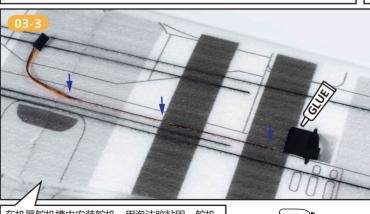
在机翼舵机槽内安装舵机,用泡沫胶粘固,舵机 线埋入预留槽内,并粘固。 Install the servo into the servo slot of the wing and fix with foam adhesive; Embed and fix the servo cable into the reserved slot. 左右相同安装。 Same installation on left and right.
