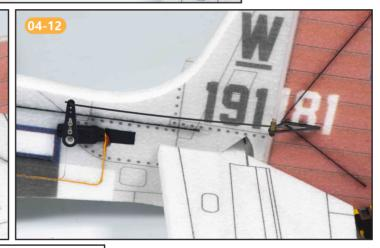
参考03-5至03-7步骤安装摇臂,舵角及连杆。 Refer to steps 03-5 to 03-7 to install the rudder arm,rudder horn and connecting rod.
