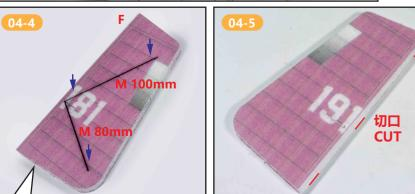
如图在垂直尾翼的背面嵌入碳片,用泡沫胶粘固。 Embed carbon sheet on the back of the vertical tail and fix with foam adhesive.
