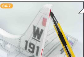
参考垂直尾翼上纸合页位置,在机身尾部切出凹槽,并安装垂直 尾翼到机身,用CA胶粘固。 Refer to the paper hinge position on the vertical tail, cut a groove at the rear of the fuselage, and install the vertical tail onto the fuselage, fixing it with CA adhesive.
