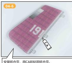
安装纸合页,用CA胶粘固纸合页。 Install paper hinges and fix with CA glue.
