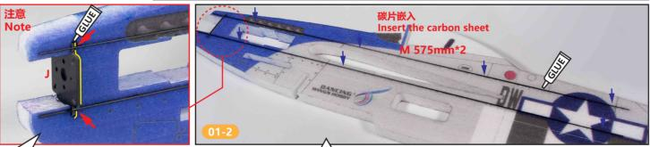
先在机头安装马达座,在预留槽埋入碳片,用涂泡沫胶 粘固,并注意碳片需嵌入马达座卡槽。 First, install the motor mount at the head, embed
