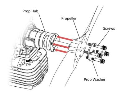
Make sure that the size of the drilling holes has correct size. The diameter of the holes is about 5.1-5.2mm.
