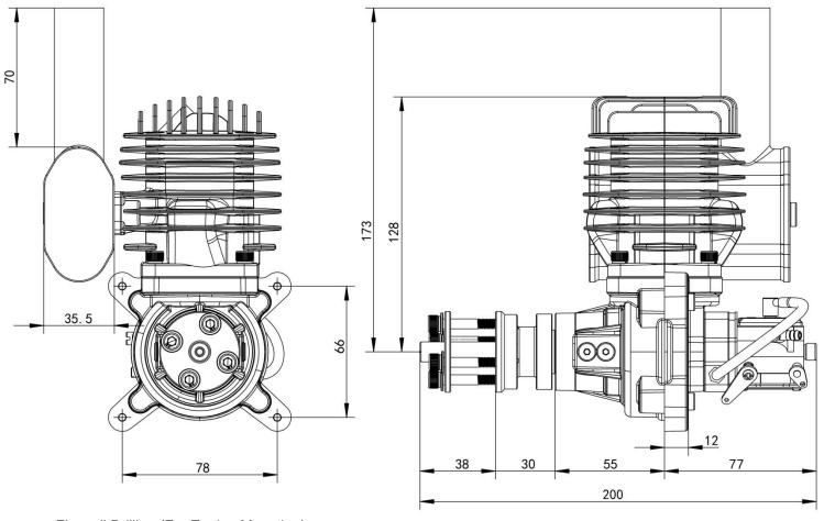
Firewall Drilling (For Engine Mounting):
