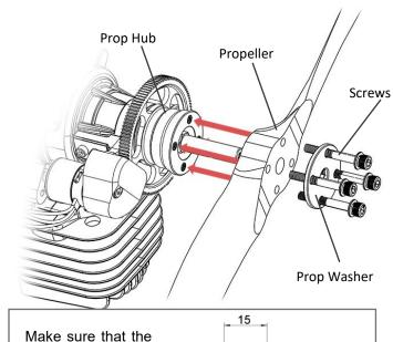
Make sure that the size of the drilling holes has correct size. The diameter of the holes is about 5.1-5.2mm.
