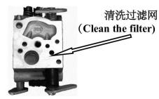
NOTICE: Please clean the fuel filter in the carburetor periodically, otherwise failure occurs with needle adjustment and the engine may work unsteadily etc.
