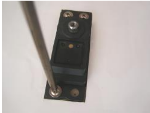
f. Using the supplied pushrod screw a ball-link onto each end.
