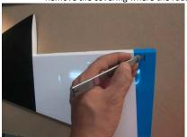
Test fit the rudder horns
