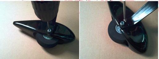
• Now line up the wheel in the centre of the wheel pant opening and tighten the collets. Remember to use nutlock and to make sure the wheel can move freely.
