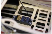
• The closed loop wires are assembled in the plane; attach the rear ball joints to the rudder. Do this to both sides.
