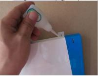
Glue the rudder horns through the rudder with CA.
