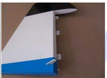
Sand the area on the horn that fits inside the rudder so the glue bonds better
