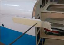
Refit the cowl and drill where the marked hole was.
