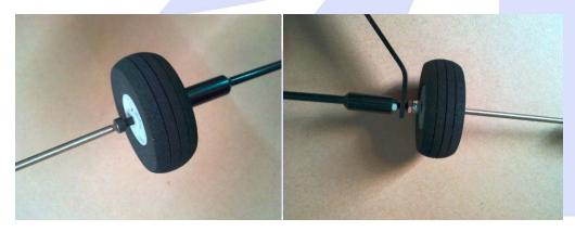
• The U/C rakes forward so use the correct wheel pant per side, and using a fine drill, drill holes for the screws.
