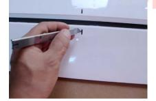
• Using sand paper rough the area that will be glued into the aileron.
