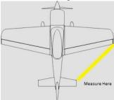
• Glueing – Once you think you are ready to glue, measure again. We recommend 2 methods for gluing. Either remove the covering on the area that is covered by the fuselage and glue with CA or epoxy, or leave the covering on and glue with thin cyno. Wicking in thin first, if a large gap is visible then use medium or thick. Remember to wick in small amounts at a time keeping the plane level, this will ensure the glue stays where it needs to be.
