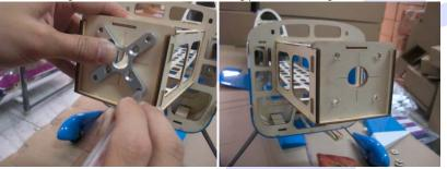
• Depending on the length of your motor you may need to use the supplied round plywood spacers to achieve the correct length for the motor.
