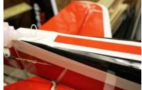
Screw the gear on with the supplied self taping screws.
