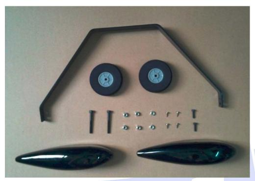
• Push each axle through the wheel holes, and tighten up with 1x self locking nut and 1x blind nut. Then pass the axle though the hole of landing gear, and tighten up with 1x self locking nut.
