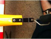
Drill a hole in the base of the rudder for the rudder steering guide.
