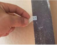
Glue the rudder hinges into both the rudder using CA. While drying use tape to keep it in alignment.
