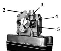
Every engine has been preset before ex-factory; it can be used directly by the customers. However, altitudes will influence the performance of carburetor, to obtain the best output of DEL engines, slight adjustment at the carburetor is very necessary.
