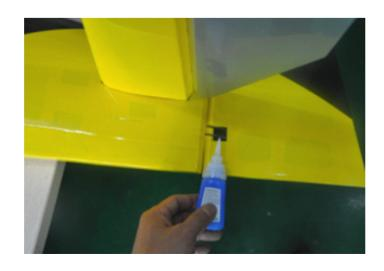
Use glue to fix up rudder horns
