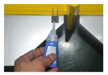
Use glue to fix up elevator horns
