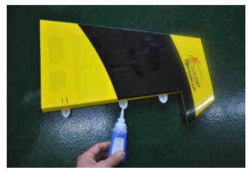
Apply epoxy into hinge hole of the rudder
