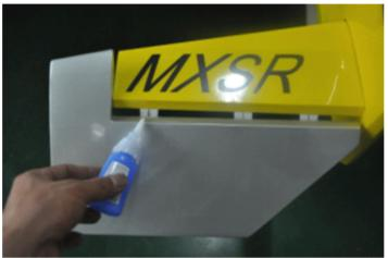
Fix up the stabilizer and elevator with hinges and AB glue.
