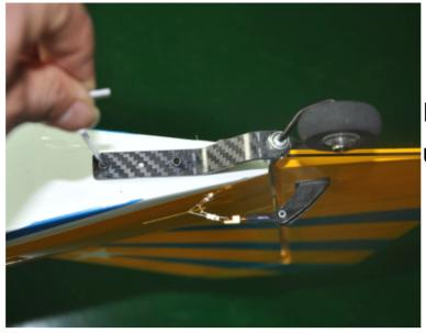
Install the tail landing gear use screws to fix up the fuselage bottom.
