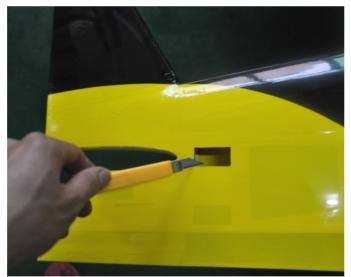
Cut the servo holes on the profile of the fuselage
