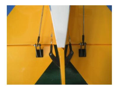
As shown in picture, This is finished for the rudder servo
