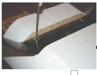
Fix up the landing gear on the fuselage bottom with screws.
