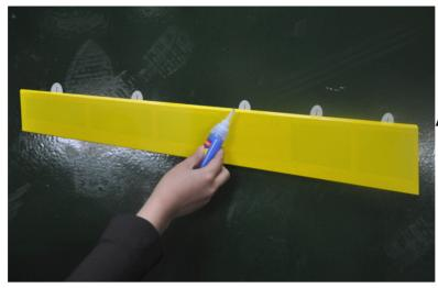
Apply epoxy into hinge hole of the wing
