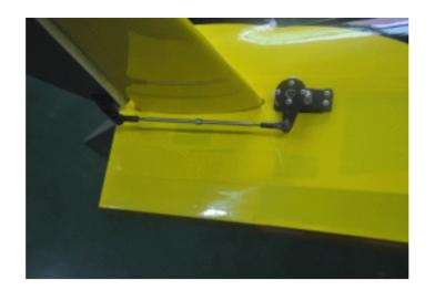
Link the servo to the elevator with pushrod.
