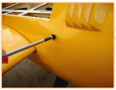
Mount the cowl using the cowl mounting screws.
