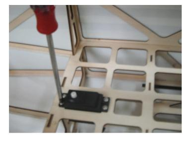
Install the rudder servo
