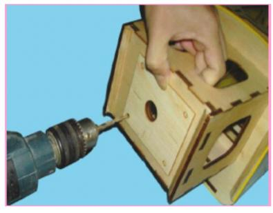
Drill the engine mounting holes as the board provided
