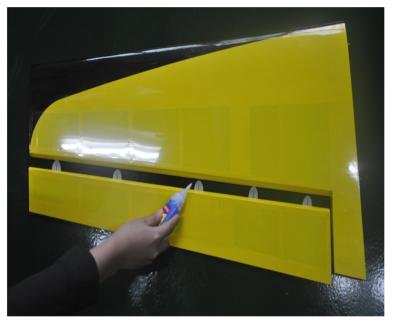
Connect the aileron and the main wing by hinges.
