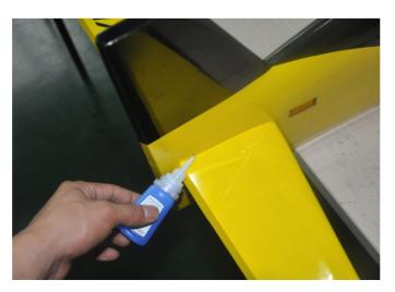
Fix up the stabilizer of the fuselage
